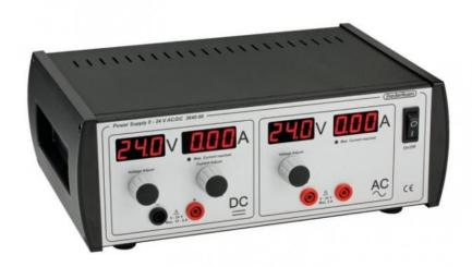
Versatile power supply for all low voltage experiments that can be used as a power generator. Four displays indicate current and voltage for each output (AC and DC). Continuously adjustable current limiter for DC. Electronic current limiter for AC.
