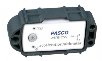
The 3-axis accelerometer / wireless altimeter, measures acceleration in all three dimensions as well as altitude to work on a wide variety of activities and experiences.
