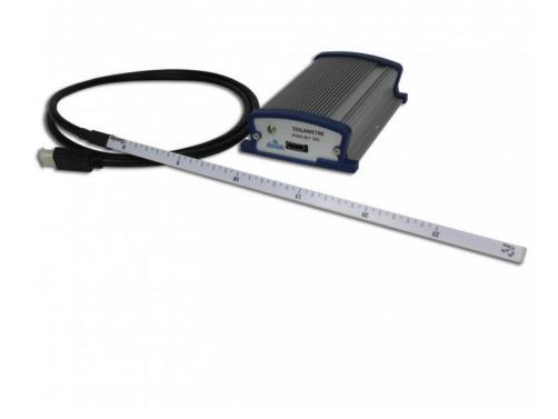
This Teslameter allows the detection and measurement of magnetic fields from 0.1 mT to 200 mT (or negative values) (field commonly created by currents from 2 to 10 A). It consists of a housing and a graduated triaxial probe for measuring 3 axes Bx, By and Bz with 3 Hall effect sensors.
