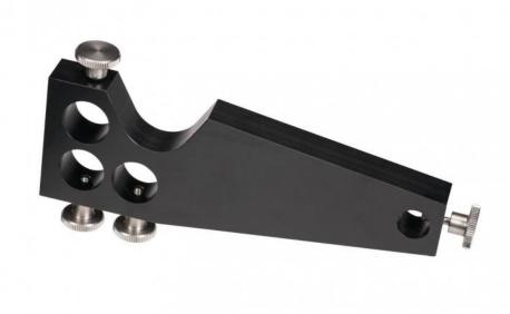
Stand for holding 3 electrodes. Three Ø 16 mm holes for electrodes. An Ø 11.3 mm hole is provided for attachment to a stand. The electrodes are held by stainless steel screws. Dimensions:  $140 \times 50 \text{ mm}$
