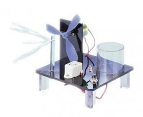
Original model for the study of vacuum - 3 different ways of revealing vacuum
