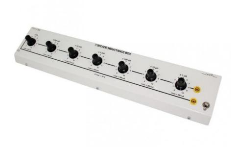
White metal box connected to a ground, with 7 rotary switches with 10 positions. The connections are made on Ø4 mm safety banana sockets.
