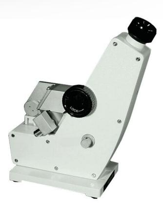
This apparatus makes it possible to determine, on two scales, the refractive index and the BRIX degree, as well as the dispersion. It is used to perform quantitative analyses of binary mixtures, concentrations of sugars, fats, etc. For liquids and solids of the type glass, plastic, etc. Refractive index: 1,3000 to 1,7000
