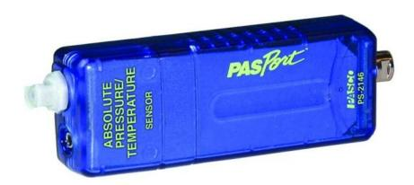
This sensor makes it possible to simultaneously or independently measure the absolute pressure and the temperature. It is supplied with a temperature sensor and a small hose and tips to connect it to the pressure sensor.
