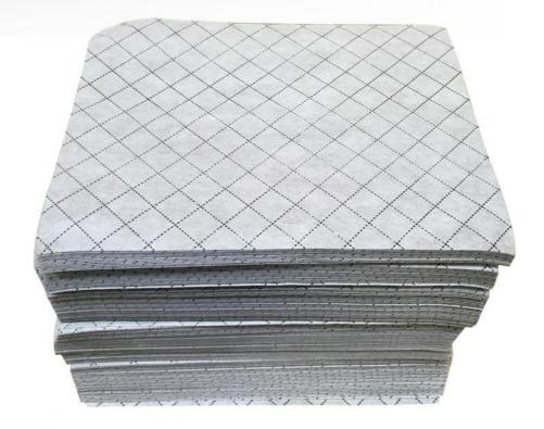
Absorbent sheets of polypropylene fiber for all liquids (chemicals, solvents, hydrocarbons ...). Absorbent single-layer, pre-cut, screened blotting paper with reinforcement sheet on one side which gives them a high resistance to friction.
