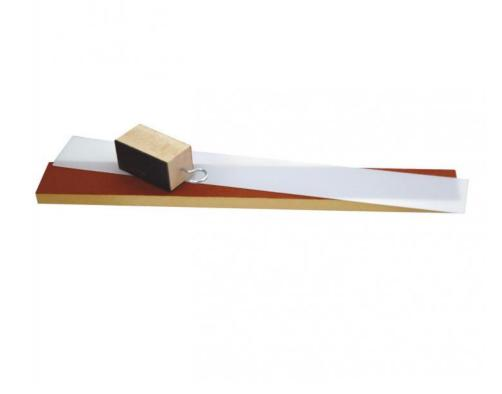
The model makes it possible to study the sliding reaction of different surfaces brought into contact with one another and thus to observe adhesion, friction or sliding.
