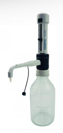
Adjustable volume dispenser, very precise, autoclavable at 121° C. Very practical thanks to its 360 ° rotating dispensing nozzle. This dispenser is very easy to clean, it comes with 5 fittings for different neck diameters of vials (25, 28, 32, 38 and 40 mm). Its manufacturing materials (PFA, FEP, PP and PTFE) give it a very good resistance to chemicals, which guarantees its shelf life without the bottle.
