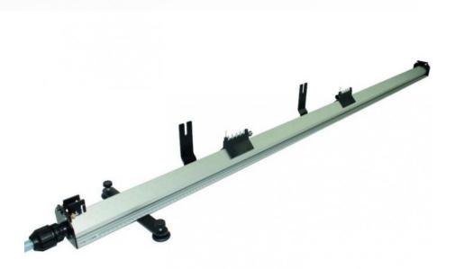
This set allows the study of one-dimensional movements without friction by the air cushion technique. A blower (to be ordered separately) injects air into a square profile aluminium track pierced with multiple small holes along its entire length. The air exiting through them allows two mobiles to move on the track while minimising friction. All accessories included with the device are delivered in a storage case. Rail dimensions: 85 x 71 x 1950 mm
