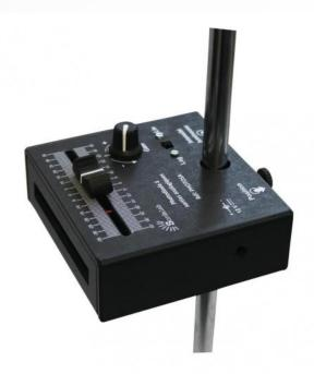
This boxed photodiode is the ideal tool to quantitatively study the phenomena of diffraction and interference. It consists of a photodiode mounted on a mobile support for moving it.
