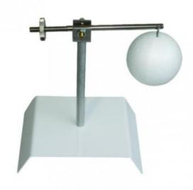
An experiment demonstrates the upward thrust that supports a body immersed in the air. The device consists of a balance beam carrying at one of its ends a polystyrene ball, and on the other a sliding weight to balance the balance. Once the vacuum is established, the atmospheric pressure exerted on the polystyrene ball disappears and the equilibrium is broken.
