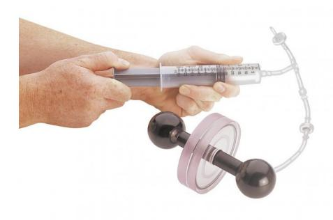
Plastic model consisting of 2 discs  $\emptyset$  97 mm x thickness 12.7 mm with gripping handle, 1 syringe with hose and non-return valve acting as a manual vacuum pump, and 2  $\emptyset$  85 and 54 mm o-rings to vary the volume between the 2 discs. Possibility of connecting a pressure sensor to the pipe.
