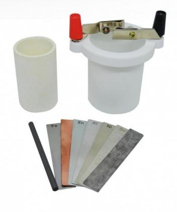
This complete kit makes it possible to study the various chemical batteries. It consists of a 65 mm diameter plastic pot, a porous ceramic vase, a set of 7 metal electrodes in strips and 1 cylindrical carbon electrode. The plastic pot is equipped with power terminals and clamps to hold the electrodes. To be completed with ionic solutions.
