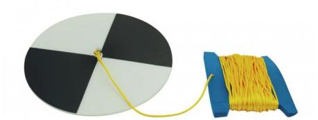
Heavy and well balanced 19.5 cm. diameter disk. Delivered with a 20 m cord for deep water measurements. Weight: 580 g.
