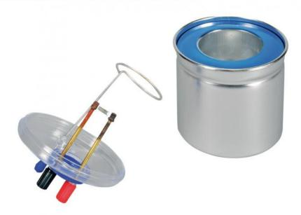
Calorimeter to determine the specific heat capacity of solid and liquid bodies, and to measure the electrical equivalent of heat.
