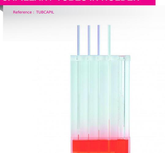
Model to illustrate capillary action, composed of 4 glass tubes of different diameters positioned in an acrylic container with a white back panel
