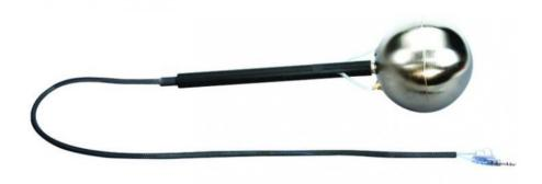
This hermetic chamber has temperature and pressure probes. Used with a pressure / temperature sensor, the chamber then makes it possible to study Charles' law: by plunging it into water at different temperatures, the pressure and the temperature of the gas at constant volume are then obtained.
