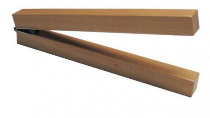
Made from two blocks of articulated hardwood, this tool produces a clean and well-defined sound. Ideal for measuring the speed of sound, the sound pulse can be recorded by microphones. Dimensions:  $27 \times 50 \times 300 \text{ mm}$
