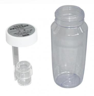
Tank to demonstrate the law of conservation of mass during a chemical reaction between 2 chemicals. For example, a piece of limestone (chalk) is placed in the bottle and hydrochloric acid in the basket suspended from the stopper.
