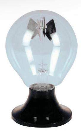
When the light rays reach the fins of the radiometer, they begin to rotate. One side of the fins is black, the other white.
