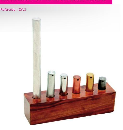
Set of 6 cylinders of identical mass but different volumes, delivered on a wooden stand.
