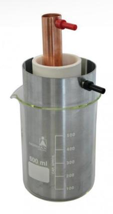
This battery has long served as benchmark standard, given its constancy and its electromotive force close to 1.10 V. Composition:
