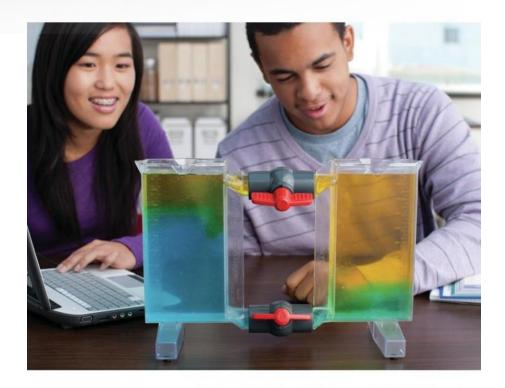
This large format model provides a better understanding of how fluid density and heat transfer are associated with fluid convection during the circulation of ocean currents.
