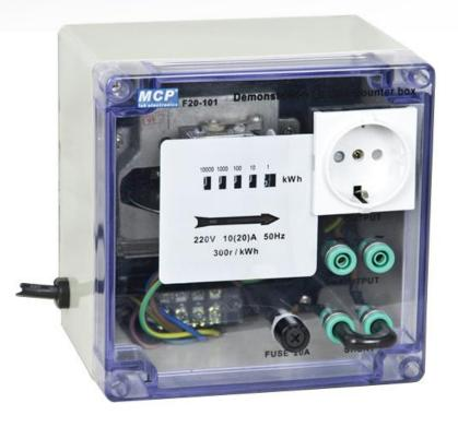
Apparatus comparable to a domestic electric meter, adapted to operate in single phase on a voltage of 220 V - 50 Hz.
