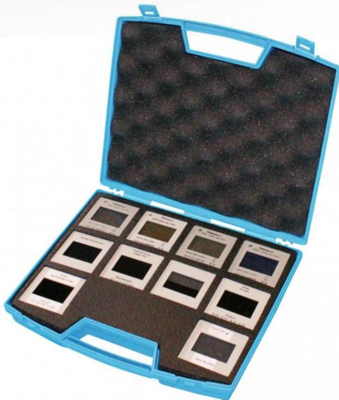
Set of 10 slides to study diffraction and interference.
