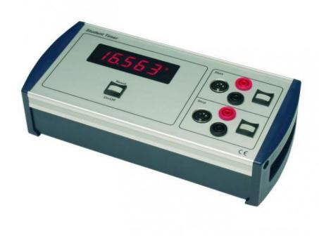
Digital stopwatch to measure freefall or air cushioning experiments.
