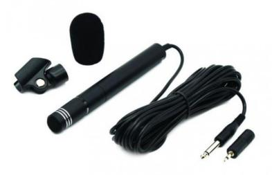
Electret multi-directional microphone with very good sensitivity. To be completed with the 12 W audio amplifier (ref AMPSON12W) for sound experiments. Impedance 1,000 $\Omega$ Bandwidth: 30 Hz to 18 kHz Sensitivity: -65 dB Ø 22 mm Length: 183 mm Connection: Ø 3.5 mm jack and adapter to 6.35 mm 1.5 V battery supplied.
