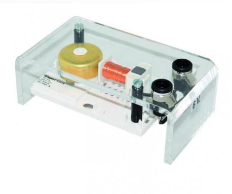
When a vacuum is created in an enclosure, the sound waves can not propagate any more, for lack of a material medium.
