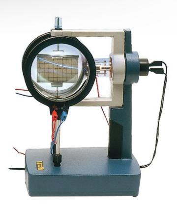
This set allows the study of electronic trajectories and their deviation in electrostatic fields created by a condenser and / or magnetic fields created by Helmoltz coils. **Réf : TUBELEC**
