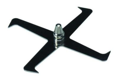
The electrostatic turnstile makes it reveal to highlight the power of the points. The accumulated charges on the points escape by ionizing the air and thus propel the arms of the turnstile which starts to turn. The propeller is placed on a needle equipped with a  $\emptyset$  4 mm plug fitting on the sphere of the Van de Graaff generator.
