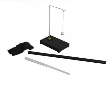
Set of accessories to perform most electrostatics experiments, fully illustrating repulsion and attraction.
