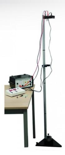
This device allows the study of free fall over a height of 145 cm.
