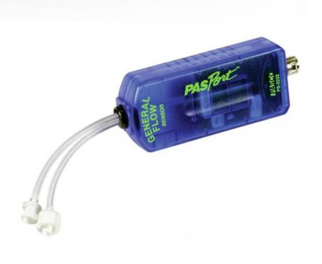
The general flow sensor determines the velocity of fluid in the air or water by measuring the pressure difference between the two inlet tubes. The Venturi tube or Pitot tube must be connected to the general flow sensor. The Venturi tube is used in a network of pipes carrying water or air. The Pitot tube is used in a free water channel or in the air.
