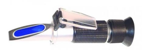
Ideal for determining the concentration of sugars in liquid medium. It tracks the consumption of glucose in a culture. This portable refractometer is a precision optical instrument With its low volume and light weight, it can be used everywhere! Model with automatic temperature compensator
