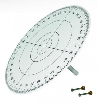
Graduated disc on rod for the study of reflection-refraction.
