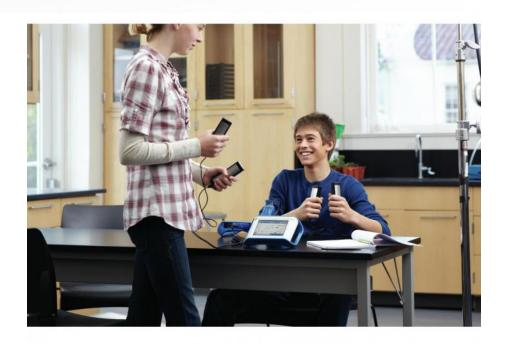
It's the easiest way to measure heart rate during exercise or at rest. The cables are long enough to allow measurements to be made while exercising. Just grab the handles with your hands to get the heartbeat. The way it works is similar to the systems found on bikes or treadmills in gyms. Electrodes located in the handles record the electrical signals emitted by the heart with each beat.
