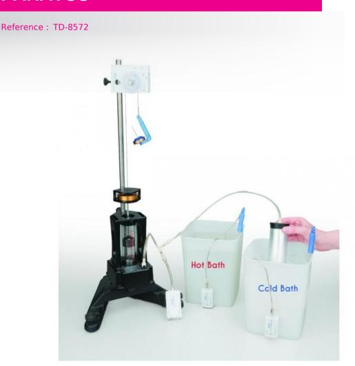
Versatile apparatus for performing quantitative experiments on the ideal gas law and the cycles of a heat engine.
