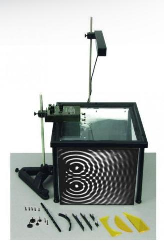
"Mechanical excitation" electromagnetic vibrator Built-in LED wave and strobe generator
