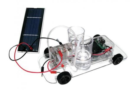
This vehicle, delivered with a photovoltaic cell, includes a fuel cell and an electrolyser. Electrolysis is done using solar energy or an external power supply. The formation of oxygen and hydrogen is visible in two water tanks. When the car hits an obstacle, it changes direction without outside intervention. This kit combines fun science with cutting-edge science.
