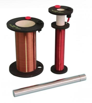
Device composed of 2 coils (inductive and induced) and a soft iron core, perfectly illustrating Faraday's experiment.
