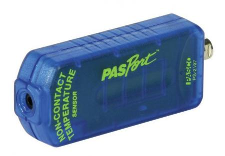
This sensor determines the surface temperature by detecting the infrared emitted. This makes it possible to measure the temperature of an object or a surface without even touching it. This allows the following applications:
