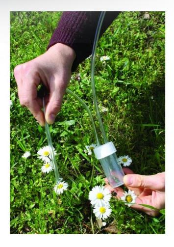
Our insect vacuum cleaner is a simple and effective solution for the capture of insects that you wish to observe. It allows to keep the integrity of the insects for more relevant observations.
