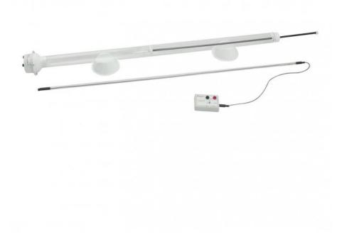
This device is ideal for resonance experiments in air columns.
