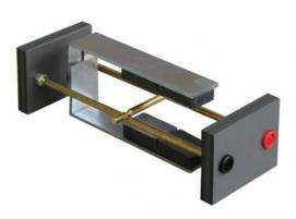
Device consisting of 2 brass rails mounted on an insulating support. When a current flows through these rails in the presence of a magnetic field (U-shaped magnet not included), a brass rod placed across the rails is then subjected to Laplace force and rolled along them.
