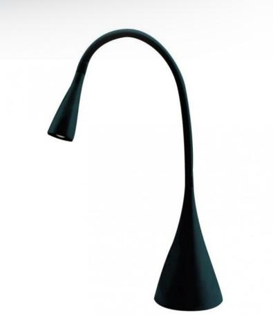
This 3W 300 lumens low voltage lamp, ideal for the laboratory, with its heavy base ensuring stability, enables lighting in all directions with its swivelling 40 cm. gooseneck Base equipped with a sensitive switch, allowing adjustment of 3 power levels. 1.7m long cable and AC adapter included. Yellow lighting. Light flow: 300 lm, Temp. : 4000K Height: 70 cm Base diameter: 11.5 cm Power: 3.0 W Weight: 1.31 kg
