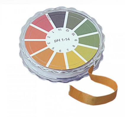
Macherey-Nagel brand pH paper (scale 1 to 14), packaged on a plastic roll for long-term stability and protection against many external factors.
