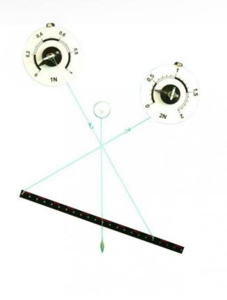
Apparatus for studying forces applied to a system at equilibrium.
